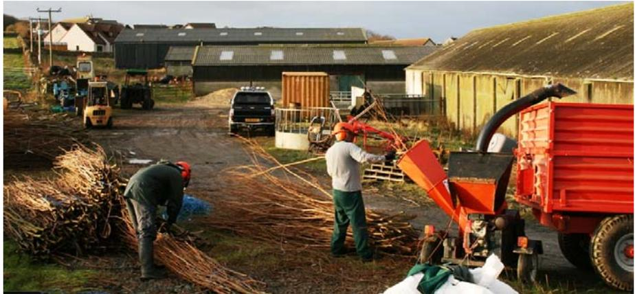
Chipping willow stems which have been dried in stacks outside to provide samples for analysis within the PELLETime project.
